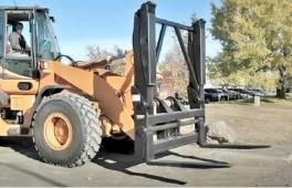
WBM Pipe and Pole Grapple is one of the most versatile of pipe grapples available. The design enables both small or large diameter pipe to be held and stabilized against the fork tines. Pipe and Pole rack widths range from 84" to 120" depending on machine size and application. Fork tines are designed in numerous sizes and configurations to satisfy lifting requirements in specific applications.
