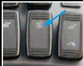
Aux hold switch: A simple push of the Aux hold switch sets and maintains the hydraulic oil flow for the implement. (All modes)
