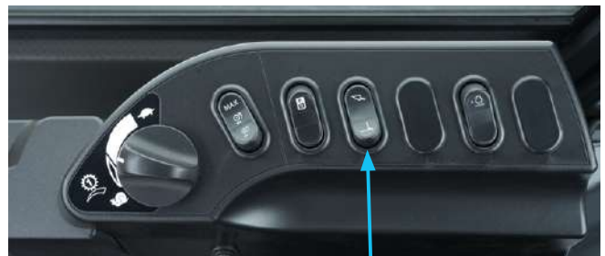
Attachment selector switch
