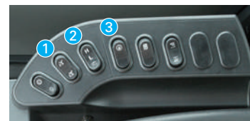
1 Dual mode engine power selection switch 2 Transmission shift mode selector switch 3 Torque converter lock-up switch
