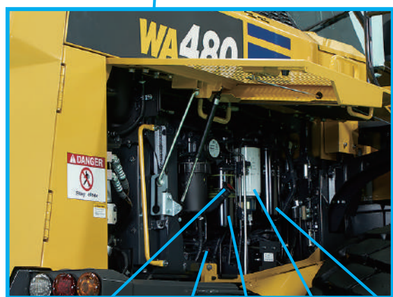
Engine oil fill Fuel filter Oil filter Engine oil dipstick Fuel pre-filter
